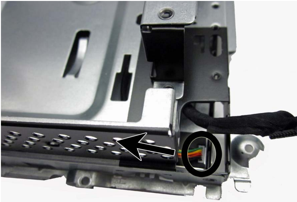
Figure 6-84 Disconnecting the backlight cable from the display panel
